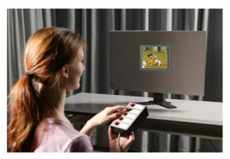
**Figure 4-1** Viewing test room at the University of Erlangen where OPTICOM conducted subjective tests. The test subject watches a scene on an adjusted TFT screen from a well defined distance. By pressing one of the keys, the test subject will be able to score the scene on the 5 point opinion scale.
