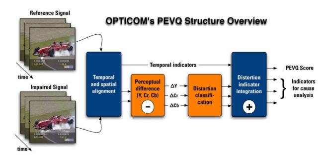
Figure 6-1 Block diagram of PEVQ
